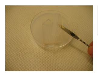
4. Cut away and remove agarose piece across the ends of all six troughs. This creates a well to drain off excess water from each channel.
