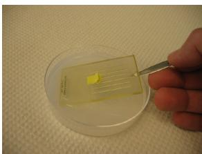
3) Slide microspatula under edge of mold and gently lift mold free of the agarose using end release notch.
